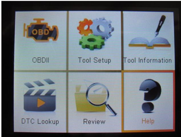
**"OBDII" should already be highlighted, so just press the ENTER button.** If it is not highlighted, then you can use the arrow buttons to move the highlight to OBDII before pressing ENTER.
